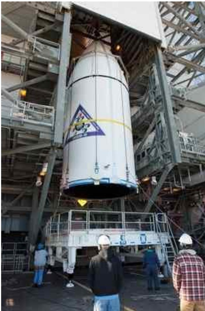
The U.S. Air Force's eighth Wideband Global SATCOM (WGS) satellite, encapsulated in a 5-meter payload fairing, is mated to a Delta IV booster at Cape Canaveral Air Force Station's Space Launch Complex (SLC)-37.
