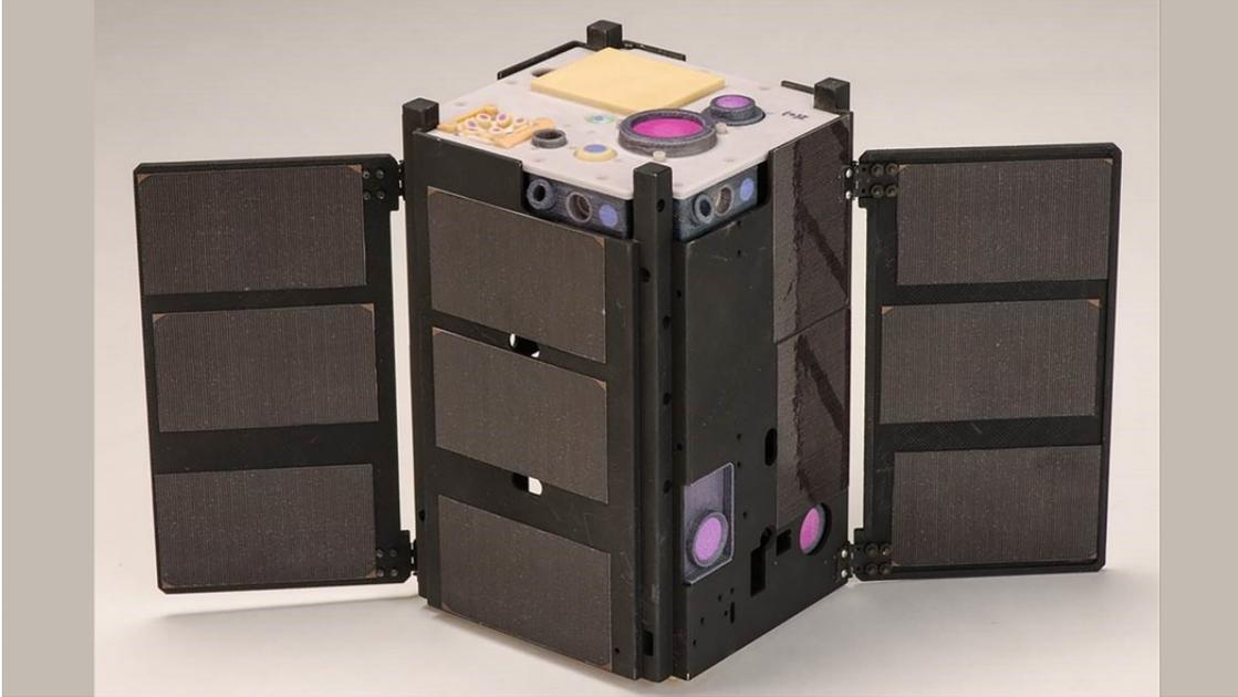
The CubeSat laser system differs from current solutions, in that it's hard-mounted to the satellite, which can be orientated as desired (Credit: NASA/Ames)
