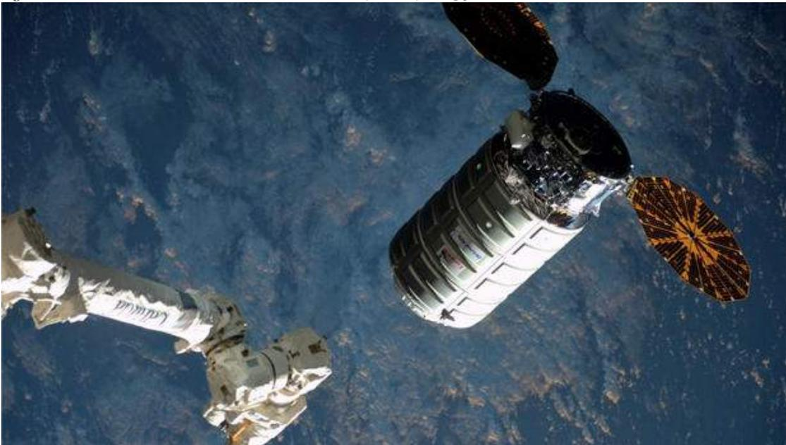
An Orbital ATK cargo ship seen moments before capture by the International Space Station's robot arm on March 26, 2016. The spacecraft plunged back into the atmosphere June 22 with a protected data recorder on board to help scientists learn more about how vehicles break apart.
